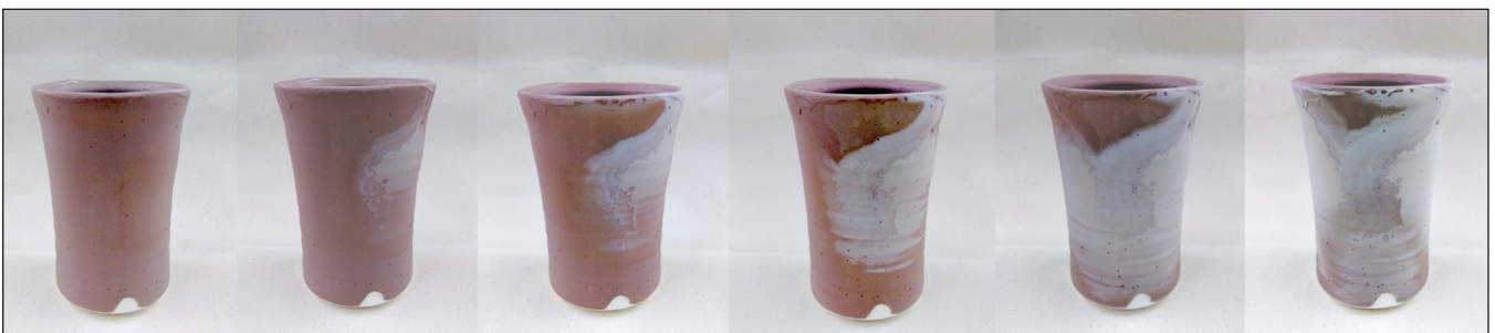
3 Salt crystals growing on the surface of the glaze as a result of drying.
