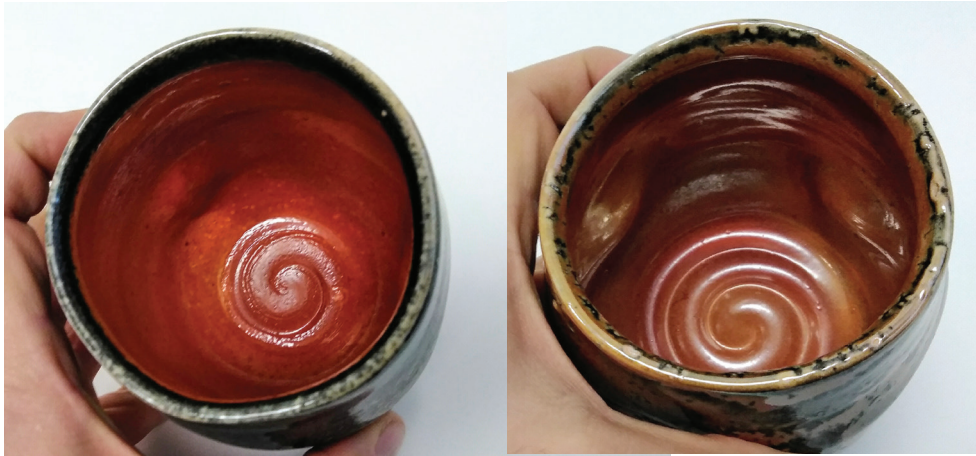
2 Liners of shino vessels (a) glazed a week prior to firing and (b) glazed immediately before loading and firing. Take note of the carbon trapping, luster, and vitrification differences.
