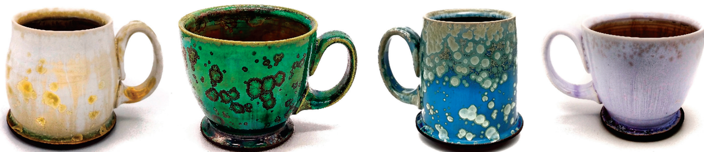
3 From left to right: The same crystalline base glaze but with 8% rutile (for gold), 4.5% copper oxide (for green), 2% cobalt oxide (for blue) (also placed in an acid bath post firing), and 7.5% neodymium (for lavender).
